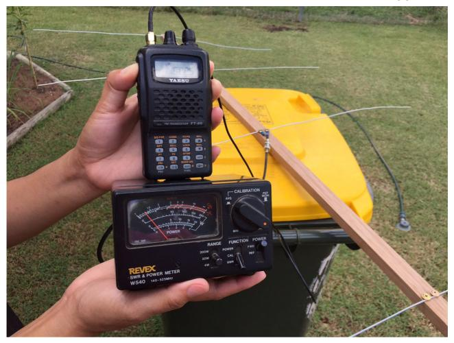
After the fine tuning was done, I programmed the FT60 to receive AM on the 2 meter band and saved the frequency in my radio with the text label of NOISE. I then went out and aimed my antenna at the electrical poles in front of my house and nothing, I had the volume up and the squelch off and all was quiet, then I walked around to the back of the house and the noise was increasing.
