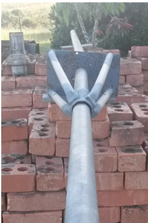
The only way was to cut it off, and adjust the legs and weld it back onto the rotator support plate.
